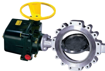
Vanessa QTL with Keystone Actuator - Quarter-turn, non-rubbing design with a unique, triple offset geometry that eliminates all seat-to-seat rubbing throughout the valve's 90° rotation.
