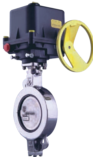
Keystone K-LOK - Double offset disc design with a variety of polymer seat materials provides high cycle bi-directional drop-tight shut-off for ANSI 150 and 300 pressure classes between flanges or as end of line service.
