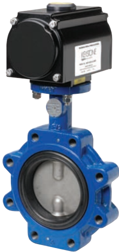
Keystone 601/602 - A heavy duty elastomer resilient seated butterfly valve, which utilizes a cartridge design seat liner for bi-directional drop-tight shut-off between flanges or as end of line service at full pressure rating.
