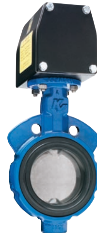
Keystone 990/920 - Thin disc profile with a triple function elastomer or polymer seat liner provides bi-directional drop-tight shut-off while isolating the valve body and stem from the line media.
