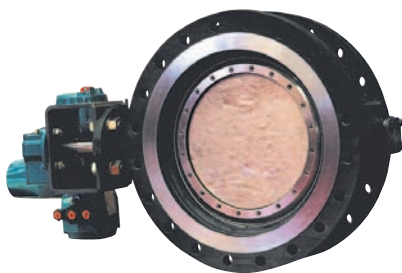
Vanessa 30,000 with Biffi Actuator - Utilizes a resilient, duplex stainless steel seal ring installed in the disc assembly to provide true zero leakage.
