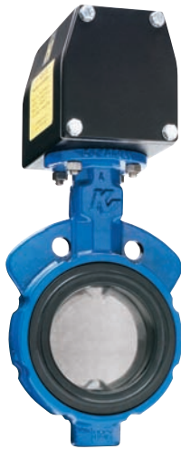
Keystone 990/920 - Triple-function seat provides bidirectional drop-tight shut-off, isolates the valve body and stem from the line media .
