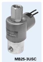
Dyna-Coil valves are used when you need to convert an electrical signal into a flow of air. 2-way models allow air to flow through the valve when energized. 3-way models allow air to flow through the valve when energized and exhaust when de-energized.
