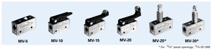
Mead's MV air switches are 3-way 1/8" ported air pilot valves that are identical in size, actuating style, and mounting characteristics to most industrial type electric limit switches. Use them in place of electric limits to save on hookup cost and eliminate spark hazard. MV valves simplify circuits by eliminating the need for wire shielding, transformers, and solenoids.
