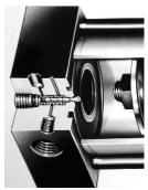
Mead's Inter-Pilot<sup>®</sup> is a miniature 3-way valve built in the cylinder head. Actuated by the cylinder's piston as it reaches the end of its stroke, the valve emits an air signal. Thus, sequencing is achieved without external limit switches and electric wiring.
