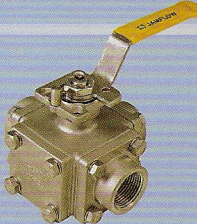
Model: #5320 Ball Valves 3-Way, Reduced Port High Neck ISO5211 Mounting Pad Material: CF8M Working Pressure: 1000WOG Size: 1/2" ~4" End Type: Threaded
