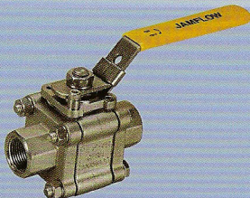
Model: #5311 Ball Valves Three Piece, Standard Port Material: CF8M Working Pressure: 1/4" ~1": 2000WOG 1-1/4" ~2": 1500WOG Size: 1/4" ~2" End Type: Threaded/Socket Weld/Butt Weld
