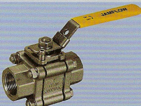
Model: #5312 Ball Valves Three Piece, Full Port Material: CF8M Working Pressure: 1/4" ~1": 2000WOG 1-1/4" ~2": 1500WOG Size: 1/4" ~2" End Type: Threaded/Socket Weld/Butt Weld
