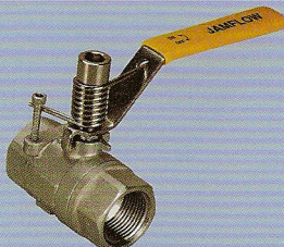
Model: #5210 Ball Valves Two Piece, Reduced Port W/ Spring Return Handle Material: CF8M Working Pressure: 2000WOG Size: 1/4" ~2" End Type: Threaded
