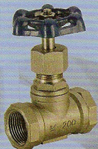
Model: #908 Globe Valves Rising Stem Material: CF8M Working Pressure: 200WOG Size: 1/2" ~2" End Type: Threaded
