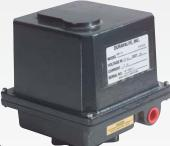
Material: Cast Aluminum Temperature Range: -40°F – 150°F Torque Range: 100–11,600 In. Lbs. Voltage: 120 VAC, 24 VAC, 24 VDC, 12 VDC and 230 VAC Available Options: Motor Brake, Unidirectional Motor, NEMA 4 and NEMA 7, Auxiliary Switches, Positioners and Other Accessories **DuraValve** is a quality supplier of brass and stainless steel ball valves, butterfly valves, pneumatic and electric actuators and actuated assemblies.
