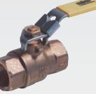
Sizes: 1/4"–1" Port Size: 1/4"–1" Full Port, Ends: NPT Threaded Ends Pressure Rating: 125 PSI Design: 2-Piece Forged Brass Body and End. Hard Chrome Plated Ball with Automatic Downstream Exhaust and Locking Handle
