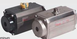
Material: Aluminum Air Supply: 40–150 PSI Temperature Range: -4°F – 175°F Torque Range: 60–12,000 In. Lbs. Finish: Available in Both Hard Anodized and Electroless Nickel Plated Design: Rack and Pinion. Double Acting and Spring Return
